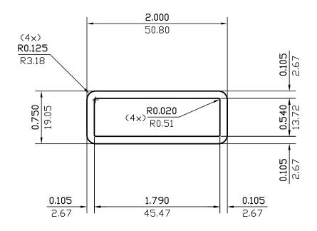
(AS SHOWN) WALL THICKNESS EXCEPT AS SHOWN DATE REV DESCRIPTION ВΥ 02/24/11 CHANGED CUSTOMER NAME J.T. 335.699 мм.2 0.520 IN.<sup>2</sup> EST.AREA EST.AREA 0.929 0.624 EST.WT. LBS/FT. EST.WT. KG/M. 9.911 251.741 EST.PER. EST.PER. MM. 5.285 134.2 OUT PER. OUT PER. MM. 2.062 52.363 C.C.D. C.C.D. 6063 FACTOR 16 M/F ALLOY & TEMP. 1:1 DWN BY C.P.SCALE DATE 01/30/2001 CKD BY
